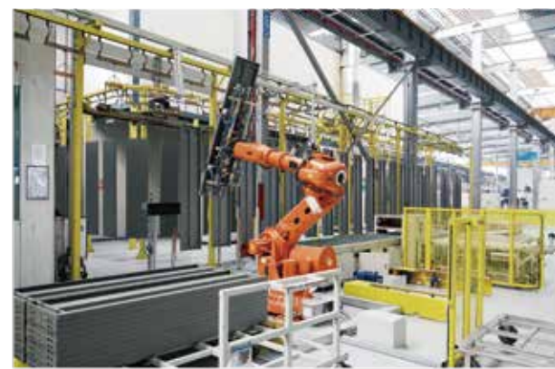
门板喷涂线 Door panels automatic painting line
