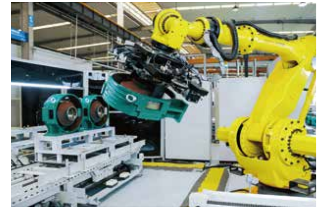
曳引机自动化装配线 Automatic assembly line of traction machine
