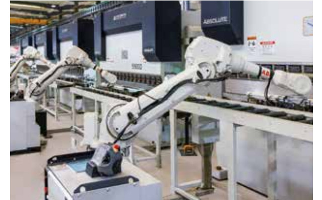
层门上坎架自动化加工线 Automatic processing line for landing door header
